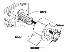
3-Inch Core Adaptors Media Hub Assembly Thumbscrews Media Supply Roll Media Hub Assembly Media Supply Roll
